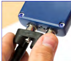
II. Remove Connectors Locking Clip (CLC)
