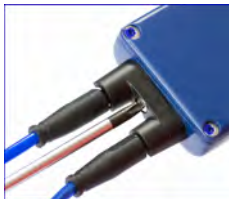
I. Unscrew Connectors Locking Clip (CLC)
